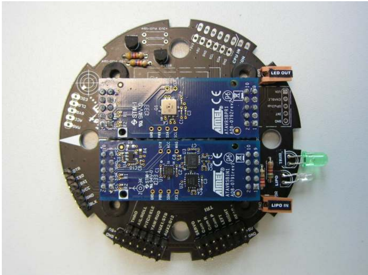
Bild/pic 23 und/and Bild 24: Flugfertiger Flightcontroller DIVIDE et IMPERA! V2 – DIVIDE et IMPERA! V2 flight controller ready for take-off
