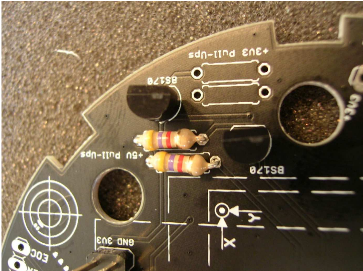
Bild/pic 17: Der fertige Logic Level Converter – completed Logic Level Converter!
